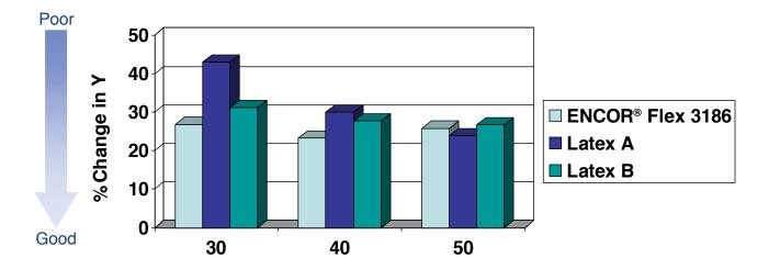
Dirt added as a slurry and allowed to dry overnight.
