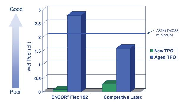
Passes ASTM D6083 wet peel adhesion requirement, even over difficult to adhere to membranes such as aged TPO, without requiring a solvent-based primer.
