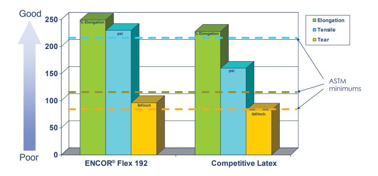
MODIFIED ACRYLIC LATEX FOR GENERAL PURPOSE ELASTOMERIC COATINGS AND SPECIALTY ROOF COATINGS
